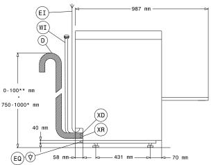
Drain ΕI Electrical inlet (power)
